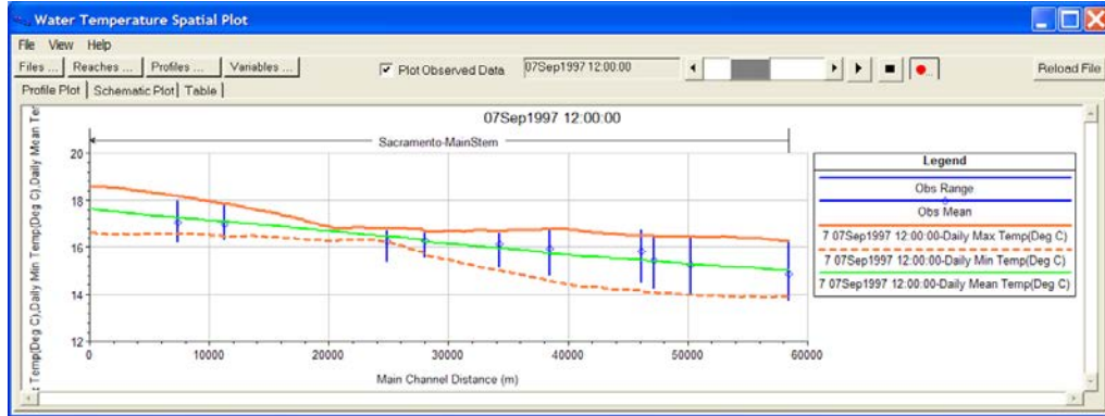
Figure 19-46. Daily maximum, minimum, and mean water temperature profile with observed data.
